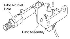
Figure 23 - Pilot Inlet Air Hole
